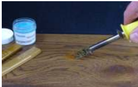
pass knife across burn-in over and over until a flat surface is achieved
