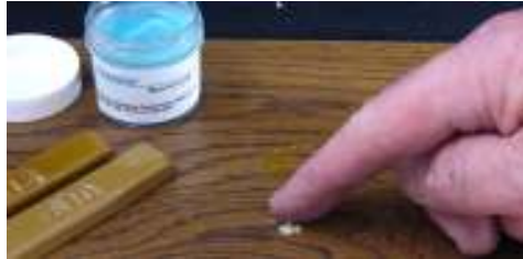
apply lube to the surrounding area of the gouge
