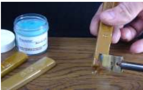
melt burn-in stick with knife, drip into the gouge
